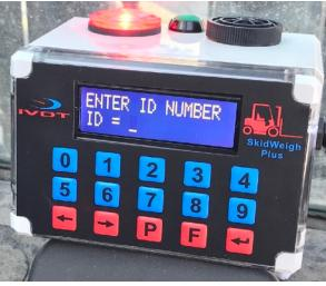
Designed to integrate seamlessly into any operation regardless of the lift truck make, model, lifting capacity or operating voltage the ED3C systems includes multiple colour lights indicating lift truck current operational status and alerts.
