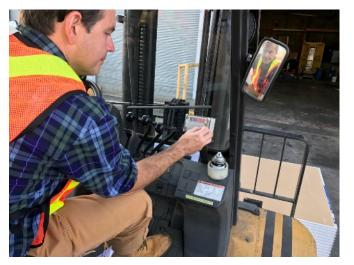
Using the **"M"** and **"Up Arrow"** buttons enter the overload weight value for your application similar to the process when calibrating the system with a load weight except the **MODE 7** digit remains throughout this operation. Once the last digit has been entered **MODE 7** will disappear.
