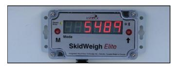
**Example:** If the lifted load is above preset overload value of 4500, in our case showing 5489 pounds the LCD display will
