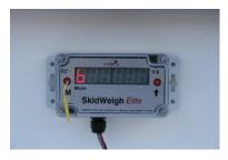
Before going to **Mode 6** please make sure that the "Known load weight" is ready to be lifted. The loaded forks must be on the ground (No hydraulic pressure in the lifting hydraulic circuit)
