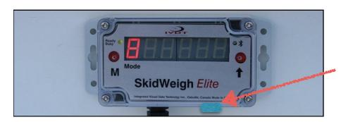
Two weighing channels switch
