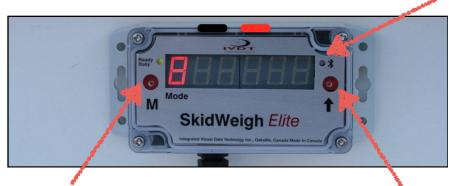
Press and hold "M" and "Arrow Up" button to pair Mobile Printer
