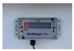
To initiate calibration press the "M" key (use a paper clip) and hold it down for approx. 5 seconds.
