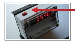
Two Weighing Channels Switch
