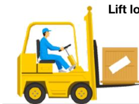
**Lift loaded forks just above the ground.** After few seconds the calibrated load weight value of 2000 will be stored in the system memory. The LCD display will prompt you to lower **“LOWER FORKS”**.
