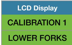
At this point you must lower the empty forks to the ground. The LCD display prompt you to input known calibration load weight.
