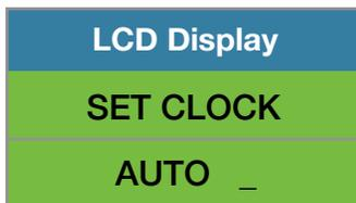
Use left ◀ and right ▶ arrow key (*bottom left side of the keypad*) to change from AUTO to MANUAL date/time set up.
