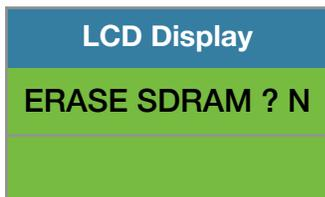
When the system has finished uploading the data to the USB memory stick the LCD display will prompt you to erase the SDRAM , all files contained on the SKidWeigh Plus ED3-UT-IM . Once you have made your selection **Y** or **N** the system will automatically bring you back to the main screen in the supervisor menu.
