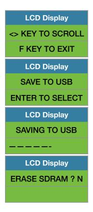
When the system has finished uploading the data to the USB memory stick the LCD display will prompt you to erase the SDRAM, all files contained on the SKidWeigh Plus ED3-EP.
