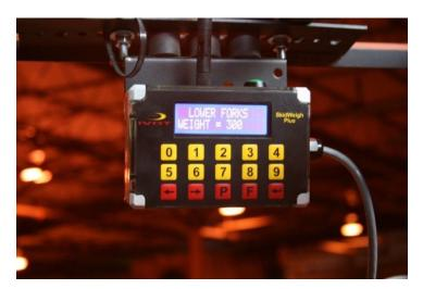
This load weight will be shown on LCD display until next time the forks are lowered to ground.
