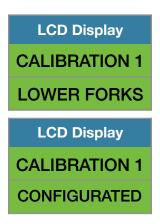
As soon the loaded forks are lowered to the ground LCD will show data / time. System is ready to be used!
