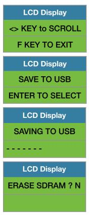
When the system has finished uploading the data to the USB memory stick the LCD display will prompt you to erase the SDRAM, all files contained on the SKidWeigh Plus ED3-IM. Once you have made your selection  $\mathbf{Y}$  or  $\mathbf{N}$  the system will automatically bring you back to the main screen in the supervisor menu.
