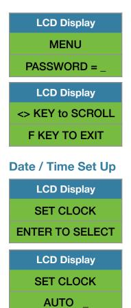
Use left ◀ and right ► arrow key (*bottom left side of the keypad*) to change from AUTO to MANUAL date/time set up.
