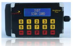
Turn ignition switch to on position The LCD display will indicate to "SCAN CARD" (as shown on the picture)
