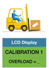
Input the overload value and press "Enter key" ←.
