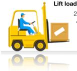
Lift loaded forks just above the ground. After few seconds the calibrated load weight value of of 2000 will be stored in the system memory. The LCD display will prompt you to lower "LOWER FORKS".
