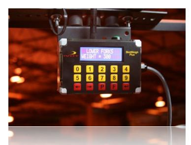
This load weight will be shown on LCD display until next time the forks are lowered to ground.
