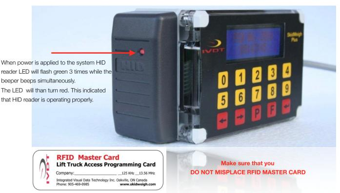
All SkidWeigh products equipped with HID RFID card reader MUST be activated with valid operator access card in order to initiate system set up, calibration and enable vehicle normal usage by authorized operator. Every system shipped out to the customer includes a **RFID MASTER CARD to be used by the end user to program any number of valid lift truck operator's HID cards.**
