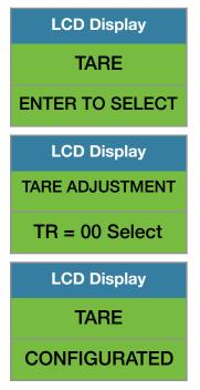
To reset or change TARE value press **F0** key and set to 0 to reset current TARE value. To change to the new TARE value, input another TARE value and press **"Enter key"** ← .
