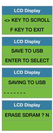
When the system has finished uploading the data to the USB memory stick the LCD display will prompt you to erase the SDRAM. Once you have made your selection  $\mathbf{Y}$  or  $\mathbf{N}$  the system will automatically bring you back to the main screen in the supervisor menu.
