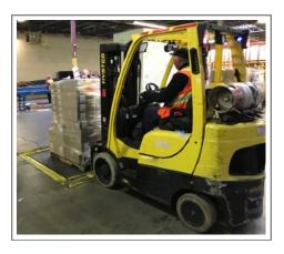
The **ED3 & ED4 SkidWeigh Plus** calibration is automatic and is done by lifting empty and loaded forks (or any other attachment such as paper clamp) **just above the ground**. MAKE SURE THAT YOU HAVE A KNOWN LOAD WEIGHT AND KEEP IT NEARBY TO COMPLETE THE CALIBRATION.
