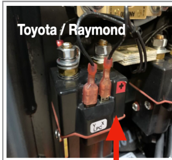
Typical Examples for two black wires lift motor pump solenoid interface
